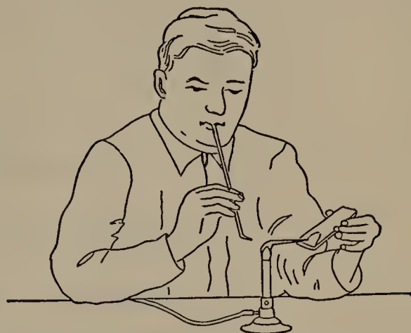
Fig. 98. Using a blowpipe flame on charcoal.
